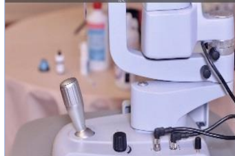
Side view of OEBC slit lamp showing the location of dimmer knob
