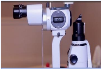
Side view of OEBC slit lamp showing the location of magnification knob
