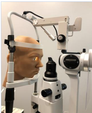
The gonioscopy model mounted in the slit lamp.
