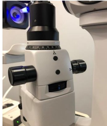
The provided slit lamp is a Zeiss-style slit lamp. Note the location of the slit height and filter thumb dials in the centre of the picture. The slit width knobs are on each side (horizontal arrow). The slit angle dial is at the top (vertical arrow).
