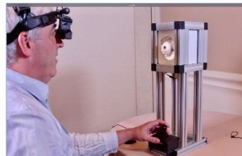
BIObot- showing the use of the joystick to control the direction of gaze
